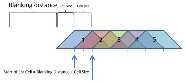
Start of 2nd Cell = Blanking Distance + 2\*Cell Size = End of 1st Cell
