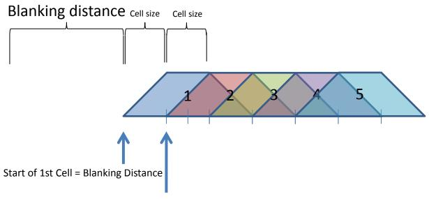
Start of 2nd Cell = Blanking Distance + Cell Size = End of 1<sup>st</sup> Cell
